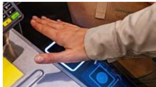
POS with Biometric Payment System (Palm Authentication)
